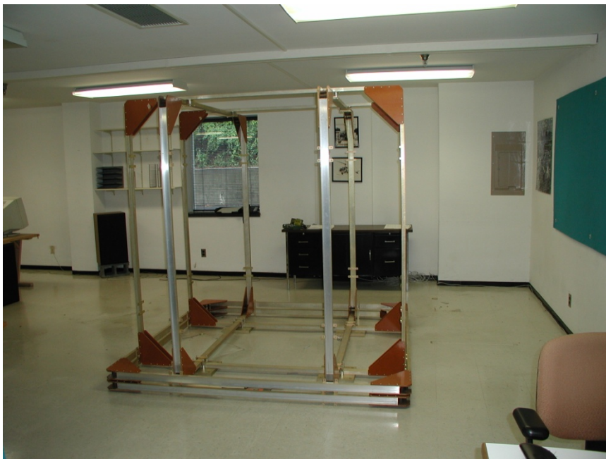
Figure 9 X and Y-axis coils in place.
