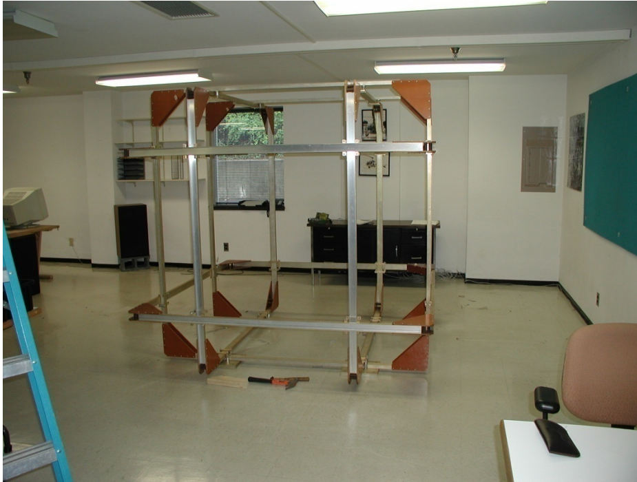
Figure 10 X, Y and Z-axis coils fully assembled.
