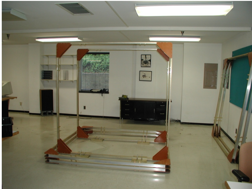
Figure 8 X-axis coils in place.
